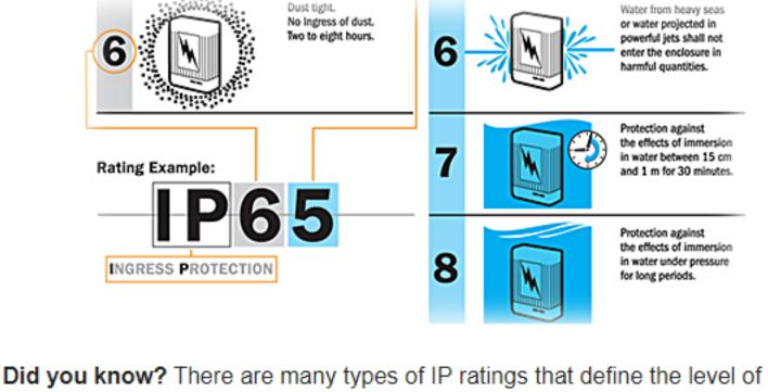
protection against solid objects (including body parts), dust, accidental contact, and water in electrical enclosures
