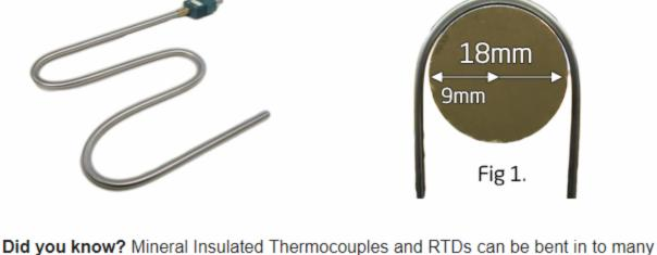
elaborate shapes. However, there is a minimum bend radius, which is 3 times the cable diameter.
