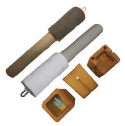
Thermal analysis cups are disposable sampling cups used in the thermal analysis of molten iron. They are placed onto a contact block which holds the cup in place. The contact block feeds back to the Digicarb/14 and readings are displayed.
