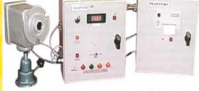
PEAKDIP is a mains powered instrument designed for use in the foundry in conjunction with a dip arm and flying lead.
