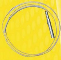
Kwik-Tip K-90 is a fast response plug-in Nickel Chromium/Nickel Aluminium type 'K' expendable thermocouple for use in non-ferrous molten metals up to 1300°C. It's fast response time means it is ideal for taking temperatures of metal in transit. Immersions per tip varies from 3 to 10 with the type of metal and slag conditions.
